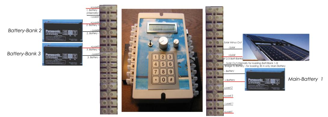
For better Performance: All Plus (Solar, Batteries etc) can be bridged external; for 30 A loading only Main-Battery: Bridge Solar out to Battery -
